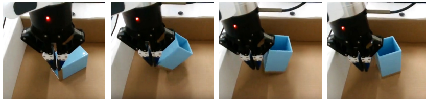
Figure 23: An example of non-quasi-static motion. The figure shows an example of executing the motion parameters to flip a mug upright. After the gripper pushes against the edge of the mug (first two images), it relies on the inertia of the mug to finish the motion which is not quasi-static (last two images).
