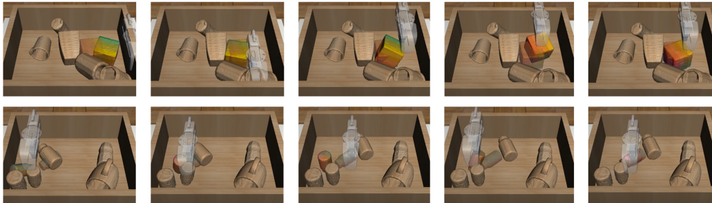
Figure 16: Qualitative results for object pose alignment tasks in cluttered environments. HACMan shows complex non-prehensile behaviors that move objects to goal poses (shown as the transparent objects). The scene objects are colored in brown to distinguish from the target object to be manipulated to the goal pose.
